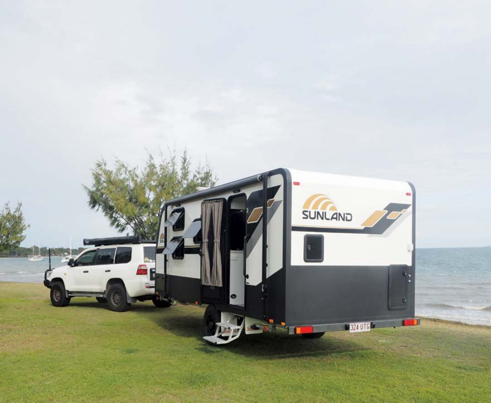
ABOVE AND BELOW The front, roof and rear walls are a single-piece composite construction; Chassis detail
